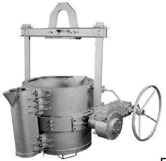
The welded-construction shell is fabricated from mild steel plate with vent holes, and reinforced with a body holding ring. The ring is welded to the shell with small wedges which create air gaps that prevent the trunnion and gearbox from being heated by conduction. The spout is welded to the shell at 90° to the trunnion position. The bail arm consists of top and side members and a hook eye plate connected by bolts.
